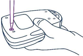
Using the screwdriver provided with the NObreath®, unscrew the screw on the back of the monitor.
